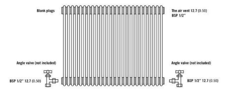
Note: Factory fitted bushes are welded in place and not removable.
